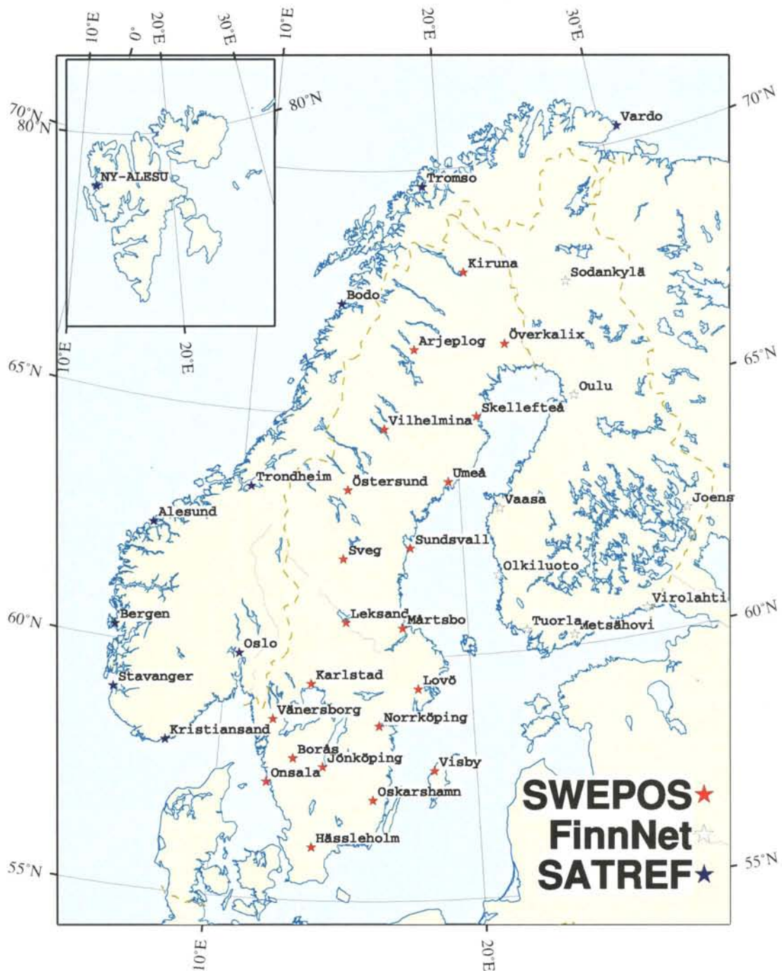
Figure 4-1. SWEPOS, the Permanent Swedish GPS Network and its Norwegian (SATREF) and Finnish (FinnNet) neighbours.
